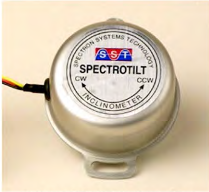
The Spectrotilt Electronic Inclinometer from Spectron features a variety of electrical interface options, fully potted electronics, EMI and ESD protection, and absolute accuracies as high as \pm 0.3 degrees.
