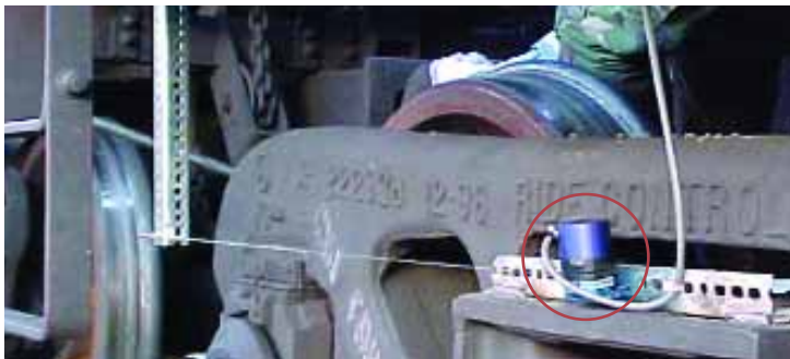
Train Suspension Monitoring
